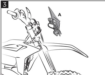
**Plug the cables and install the Acerbis headlight mask (A).**
