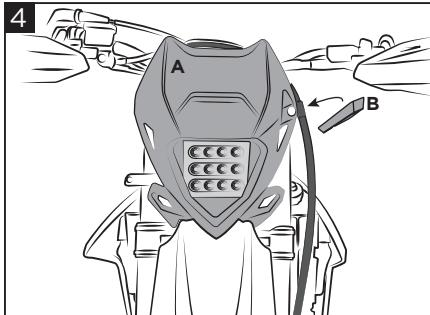
**Place the cable entry (B) in the proper place.**
