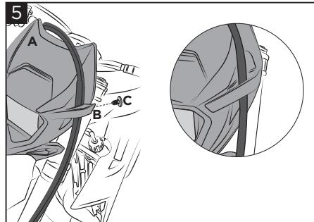
**Place the cable in the cable entry (B) and reassemble the latter using the screw (C).**
